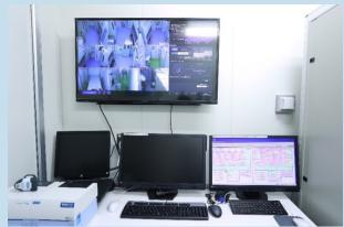
An advantage of the monitoring system allows history data to be traced back. If there is a malfunction in a refrigerator, checking the change in chamber tempera-ture from the time the malfunction occurs to when the alarm sounds allows the person in charge to take appropriate post-accident actions for the stored items.
