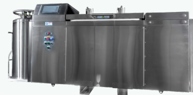
High Capacity Controlled Rate Freezer Up to 781-Liter Capacity
