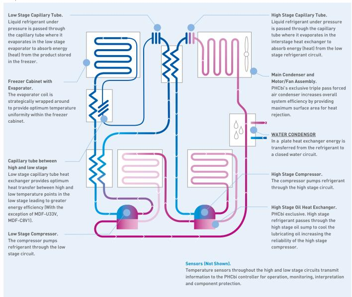
Ultra low temperature refrigeration systems can be extremely demanding with high operating pressures, increased temperatures and stresses and adverse effects on lubricant oil.
